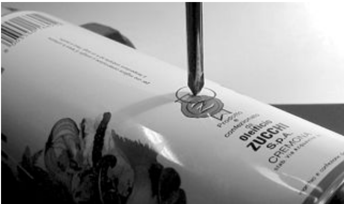
Figure AC 23: Mark the hole before drilling.
