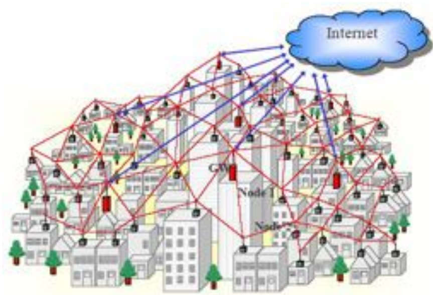
Figure MN 1: A metropolitan area mesh network, providing local connectivity and Internet access via multiple Internet gateways
