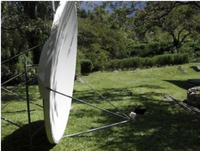
Figure CsLD 4: 2.4 m offset fed reflector with a 12 dBi antenna at its focus, looking 14^\circ down. The actual elevation is 8^\circ up.
