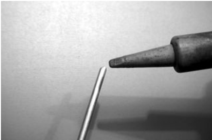
Figure AC 25: Tin the end of the wire before soldering.
