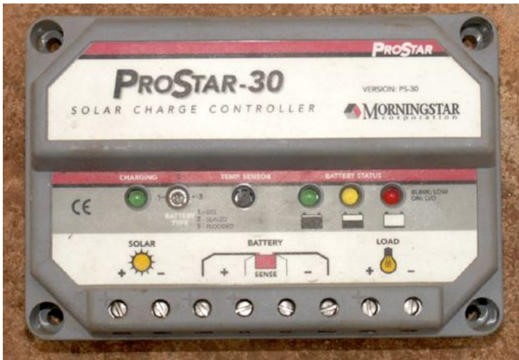
Figure OGP 3: A 30 Amp solar charge controller
