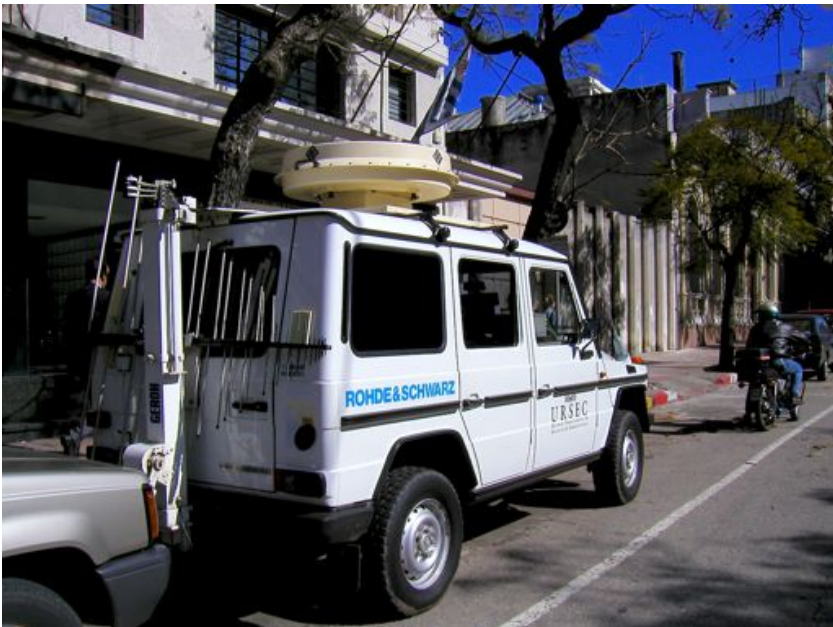
Figure RS 2: A special vehicle for spectrum monitoring in Montevideo, Uruguay.
