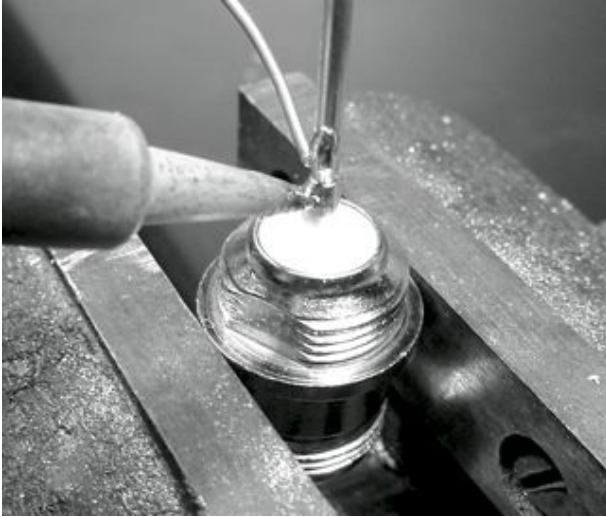
Figure AC 26: Solder the wire to the gold cup on the N connector.
