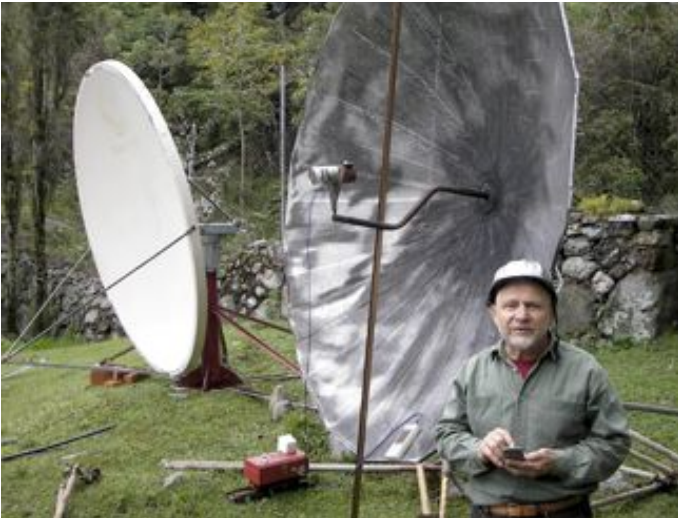
Figure CsLD 6: Finding the focus of the antennas with the 2.4 GHz feed
