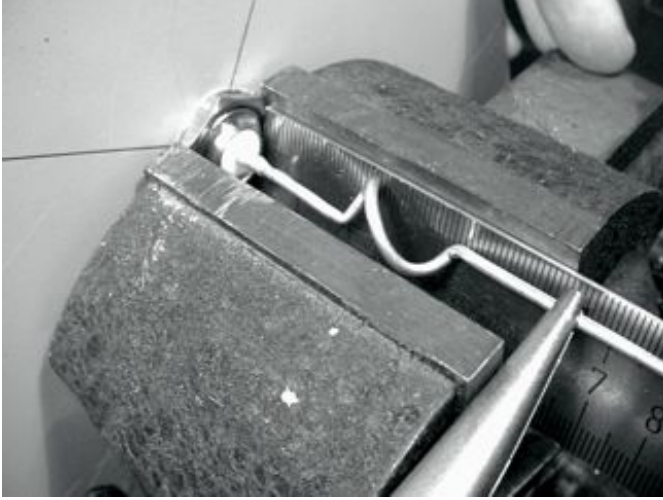
Figure AC 15: Stretching the coils. Be very gentle and try not to scrape the surface of the wire with the pliers.
