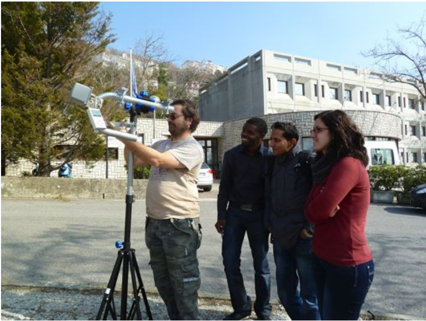
Figure RS 6: Participants from Albania, Nepal, Malawi and Italy testing an antenna with the RF Explorer Spectrum Analyzer in Trieste, February 2012.
