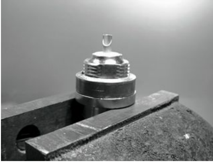
Figure AC 11: Adding a copper pipe spacer helps to match the impedance of the antenna to 50 Ohms.
