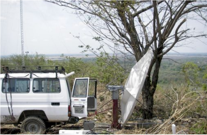
Figure CsLD 9: El Baúl antenna installation. Actual elevation was 1° upward, since the antenna has an offset of 22.5°.
