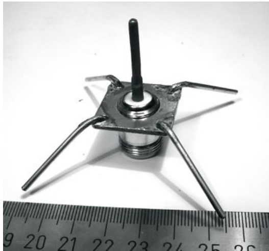
Figure ATL 11: Quarter wavelength ground plane antenna.
